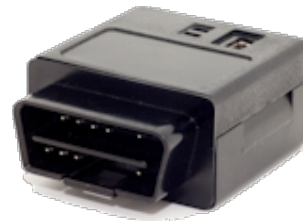
Figure 2: Our TCU showing both the OBD-II and USB connectivity.
